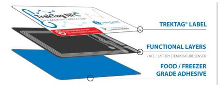
TrekTag® NFC is a temperature data logger designed to accurately record temperature data over time. This data can be used to indicate if a product has remained in the desired temperature range during storage or transport. Data can be reviewed from TrekTag® Mobile Application and be sent to TrekTag® Analytics "cloud" for further analysis.
