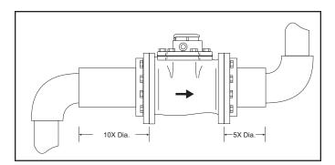
**Flanges.** The WJ meter is compatible with any standard 150 lb. ANSI drilling, flat or raised face. Take care that gaskets (included) do not protrude into the meter due to misalignment. Adhering the gasket to the meter flange with gasket adhesive is a good practice that will aid installation.
