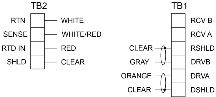
Figure 2-11: Wiring for Rosemount 1066 transmitter
