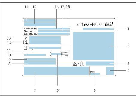
**₽** 1 Example of a transmitter nameplate
