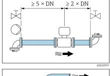
Keep a sufficient distance to the next pipe elbow.
