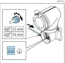
1. Loosen the Allen key of the securing clamp.
