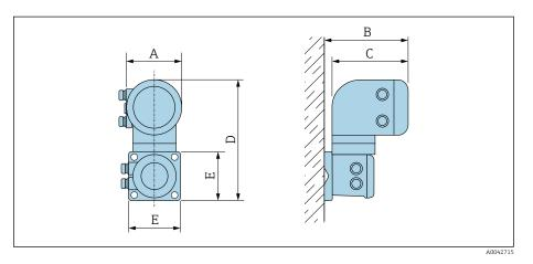
A 1) С Е Order code for "Housing" D [mm] [mm] [mm] [mm] [mm] Option P "Remote, aluminum, coated" 139 185 178 309 130
