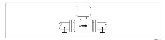
20 Potential equalization via measuring tube
