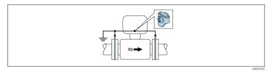
22 Potential equalization via ground terminal and ground disks
