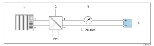
■ 12 Connection example for 4-20 mA current output (passive)
