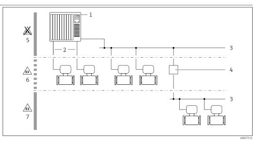
I Possibilities for integrating measuring devices into a system
