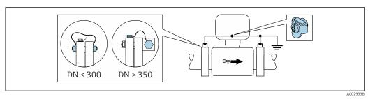
21 Potential equalization via ground terminal and pipe flanges
