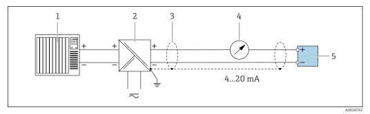
☑ 3 Connection example for 4 to 20 mA HART current output (passive)
