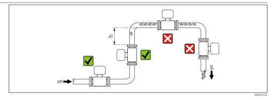
Preferably install the sensor in an ascending pipe, and ensure a sufficient distance to the next pipe elbow:  $h \geq \ 2 \times DN$
