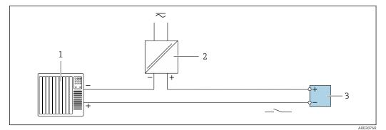
■ 17 Connection example for relay output (passive)
