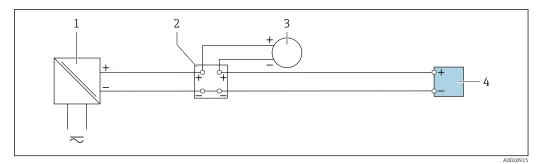
■ 18 Connection example for 4 to 20 mA current input
