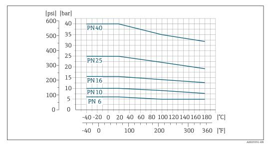
28 Process connection material: stainless steel, 1.4571 (F316L)
