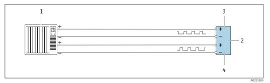
■ 15 Connection example for double pulse output (active)
