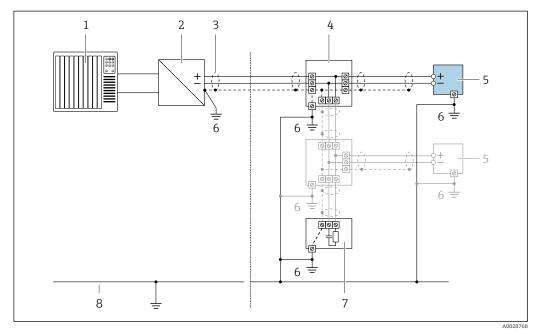
Connection example for FOUNDATION Fieldbus
