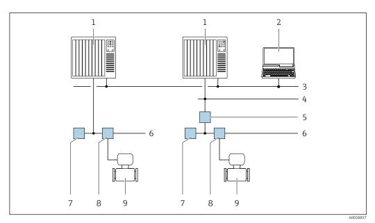
■ 46 Options for remote operation via FOUNDATION Fieldbus network
