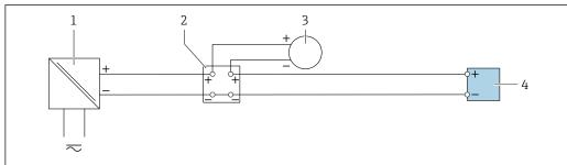
€ 18 Connection example for 4 to 20 mA current input
