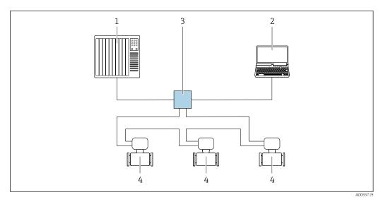
3 Options for remote operation via PROFINET network: ring topology
