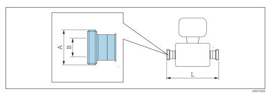
Length tolerance for dimension L in inch:  $\pm 0.06\ /\ -0.08$
