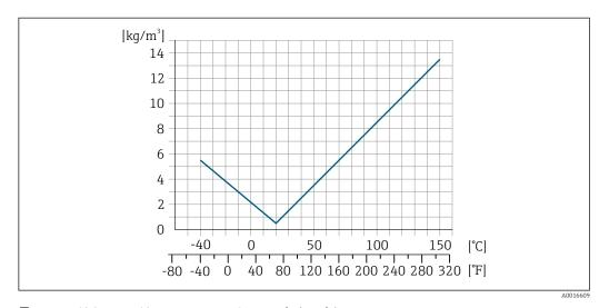
■ 20 Field density calibration, for example at  $+20 \,^{\circ}\text{C}$  ( $+68 \,^{\circ}\text{F}$ )
