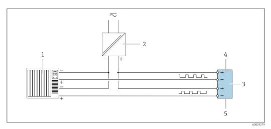
Connection example for double pulse output (passive)
