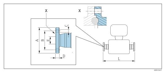
■ 34 Detail X: Asymmetrical process connection; the part shown in blue is provided by the supplier.
