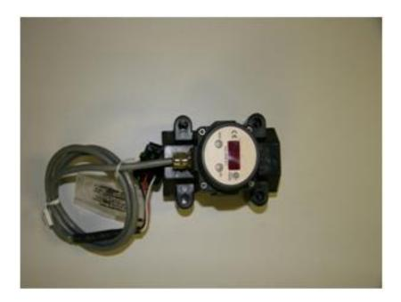
Complete unit as shipped including flowmeter and cabling.
