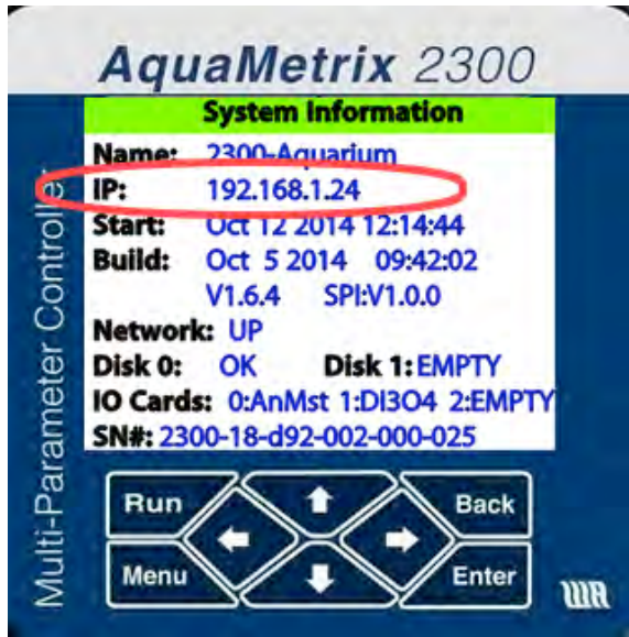
Figure 2-5 - The IP address of the 2300 assigned by the router is listed on the second line.
