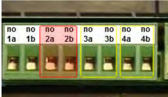
Figure 6-12 - Relay connections on the back of the 2300. The red shaded rectangle shows the relay chosen in the Wizard.
