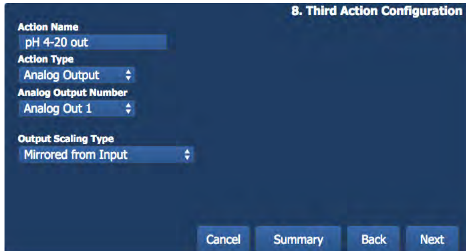
Figure 7-5 – With the analog output card installed
