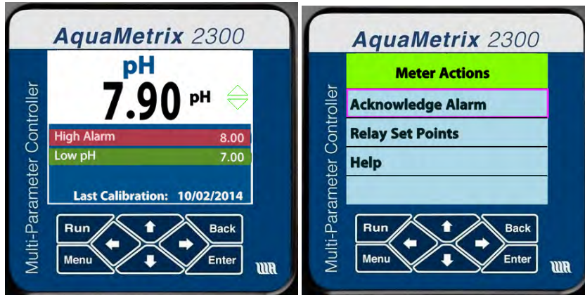
Figure 6-10 - The bar around the High Alarm alert flashes red until you press the Enter button. Pressing the Enter button on the Meter Actions screen brings you back to the screen on the left—only this time with a steady red bar.
