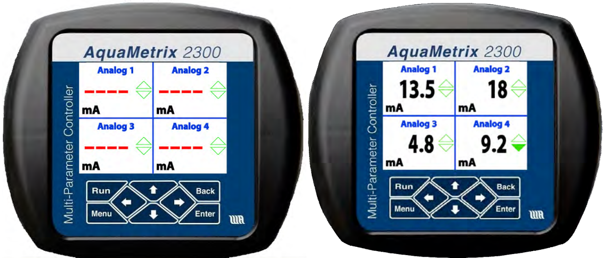
Figure 3-2 – The 2300 comes preconfigured to start working without the web-based configuration that still has to be done. The RUN screen showing four analog probe inputs. On the left is a display showing that no probes have been connected. On the right, four analog probes have been connected.
