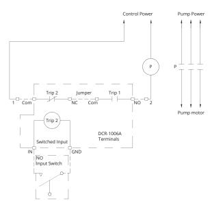
DCR Switched Input as E-Stop Control Wiring
