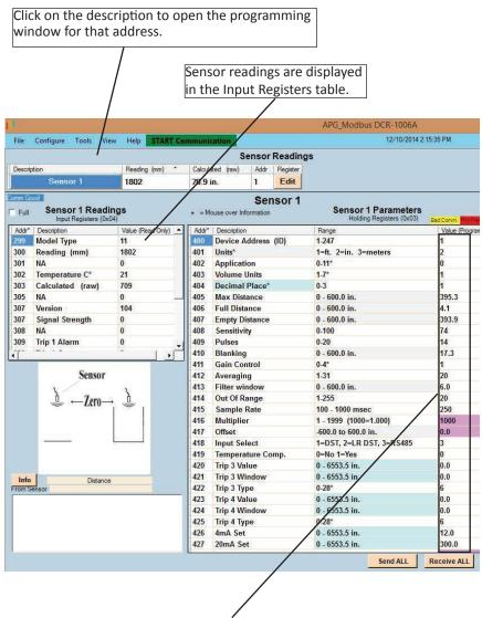
The register values should automatically populate. If not, click "Receive All" to retrieve the register values from the sensor.
