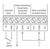
Trip 1 (NO) is controlled by the sensor (see Relay Trip Types and Relay Logic Diagrams on pages 32-33), closing for ON conditions. If the NO input switch closes, Trip 2 will open, breaking the circuit through Trip 1.
