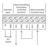
Trip 1 (NO) is controlled by the sensor (see Relay Trip Types and Relay Logic Diagrams on pages 32-33), closing for ON conditions. Since Trip 2 is also NO, both trips must be active (ON) for the Pump/Valve circuit to be complete.
