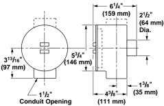
① All NEMA 7/4 rated terminal enclosures supplied with a gasket for the cover.
